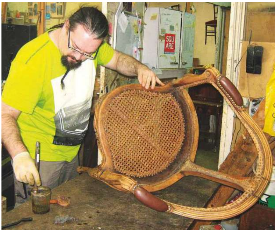
This chair is being laboriously and carefully cleaned to preserve the patina using an organic specialised wood stripper
